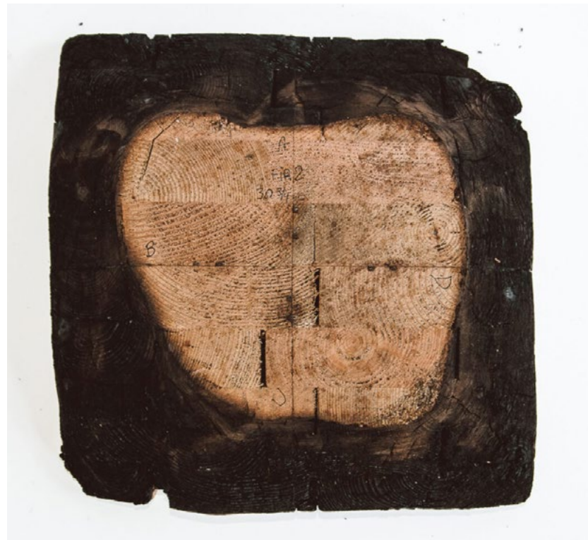
3-HR Rated Glulam Column from Timber Lab
